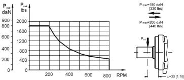
Radial Shaft Load Prad for C,CO Shaft Extensions by L=30mm[1.81in]
