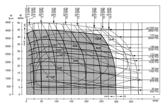
The function diagrams data is for average performance of randomly selected motors at back pressure  $5+10 \text{ bar } [72.5\div145 \text{ PSI}]$  and oil with viscosity of  $32 \text{ mm}^2/\text{s} [150 \text{ SUS}]$  at  $50^{\circ}\text{C} [122^{\circ}\text{F}]$ .
