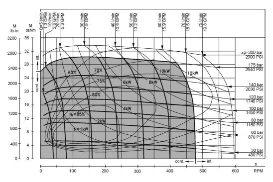
The function diagrams data is for average performance of randomly selected motors at back pressure  $5+10 \text{ bar } [72.5\div145 \text{ PSI}]$  and oil with viscosity of  $32 \text{ mm}^2/\text{s} [150 \text{ SUS}]$  at  $50^{\circ}\text{C} [122^{\circ}\text{F}]$ .
