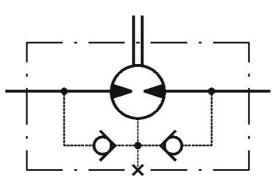
The shaft seal pressure equals the pressure in the drain line
