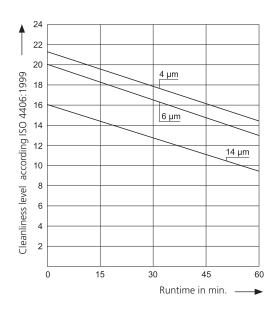
D2: FA2 016 with 10µm EXAPOR®MAX filter element
