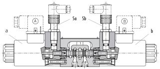
**Spool Speed Control** in millimeters (inches)
