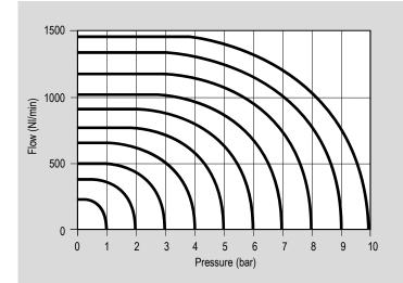
Mechanical operated valves series AC 1/8", 3/2 Normally closed, with plunger
