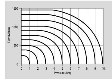
Mechanical operated valves series AC 1/8", 5/2 Spring return, with plunger
