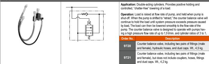
**CAUTION:** The 9720 patented counter balance valve has a pilot pressure as high as 210 bar. Because this pressure is applied to the rod end of the cylinder while it is already under load, the system should not be sized for loads greater than 80% of cylinder rated capacity. To prevent sudden, uncontrolled descent of a load as it is being lowered, use a 9596 Load-Lowering Valve or 9720 Counter Balance Valve in conjunction with the directional valve used in your application.
