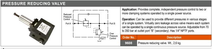
A CAUTION: Over Pressure control must be set at a higher value than operating pressure.
